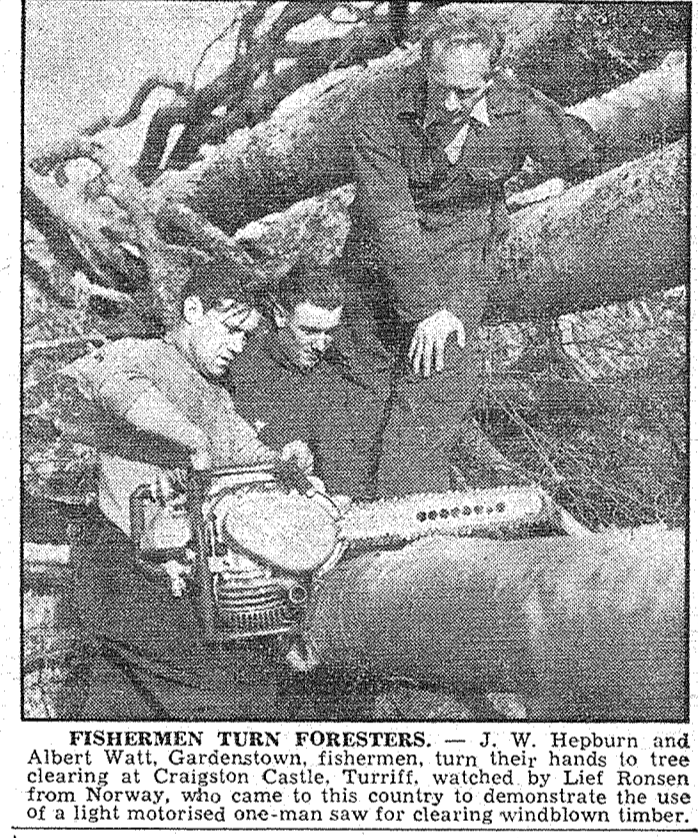
FISHERMEN TURN FORESTERS.—J. W. Hepburn and Albert Watt, Gardinstown, fishermen, turn their hands to tree clearing at Craigston Castle, Turrieff, watched by Lief Ronsen from Norway, who came to this country to demonstrate the use of a light motorised one-man saw for clearing windblown timber.
